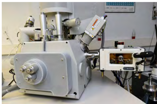
Fig. 26. Environmental Scanning Electron Microscope (ESEM) with SE, BSE detectors and EDS system at the CIC-UGR.
