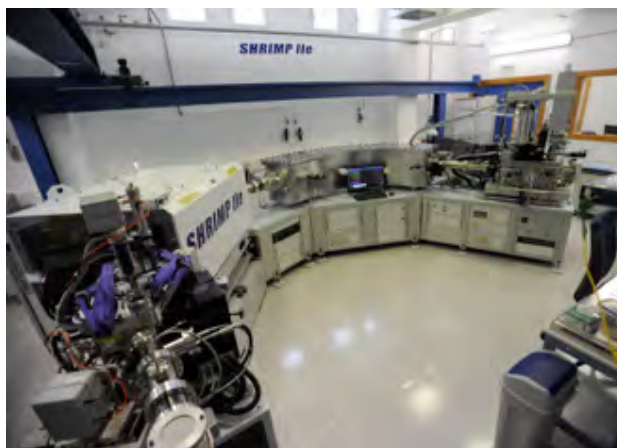
Fig. 30. Sensitive High-Resolution Ion Microprobe (SHRIMP) at the CIC-UGR.
