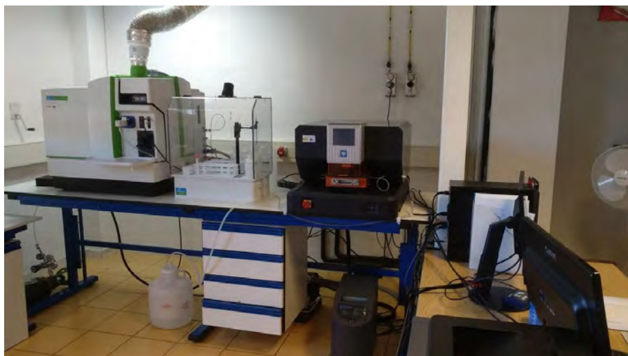
Fig. 29. Laser Ablation Inductively Coupled Plasma-Mass Spectrometry (LA-ICP-MS) with New Wave Research NR 213 laser ablation system at the CIC-UGR.
