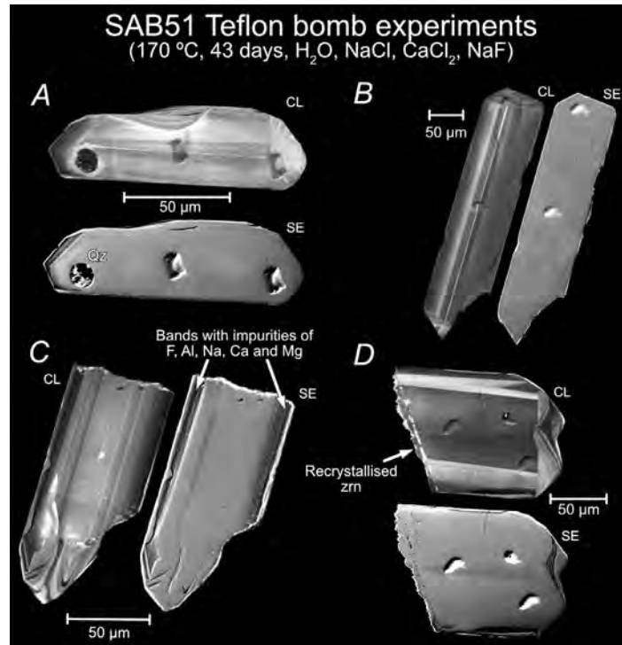
Fig. 49. SE and CL images of low- T leaching experiments from zircons of tonalite SAB51. A) Zircon grain from H 2 O leaching experiment (run Z-2) that appears zoned with alternating light-gray and dark-gray bands parallel to the longest axis. B) Zircon grain from NaCl leaching experiment (run Z-4), that appears zoned with alternating light-gray and dark-gray bands parallel to the longest axis. C) Zircon grain from CaCl 2 leaching experiment (run Z-6), that appears zoned with alternating light-gray and dark-gray bands parallel to the longest axis. These bands present impurities of F, Ca, Na and Mg. D) Zircon grain from NaF leaching experiment (run Z-8); very thin band roughly parallel to a fracture surface of a split grain with abundant micropores and luminescent zircon.
