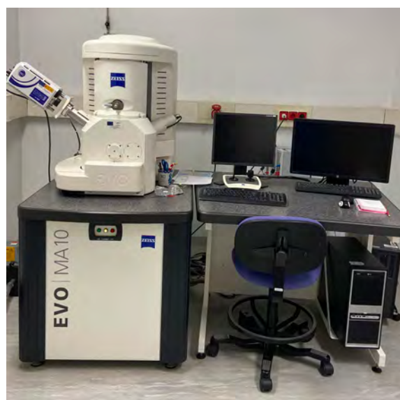
Fig. 27. Scanning Electron Microscope (SEM) with BSE, SE, CL and EDAX detectors at the CIC-UGR.
