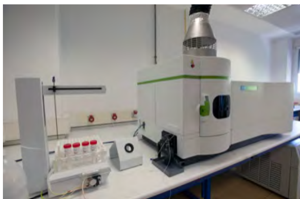
Fig. 31. Inductively Coupled Plasma Optical Emission Spectroscopy (ICP-OES) with automatic sampler PERKIN-ELMER S10, at the CIC-UGR.
