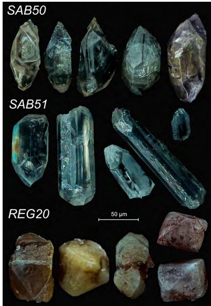
Fig. 11. Macro-photographs of untreated zircon grains from orthogneiss SAB50, tonalite SAB51, and syenite REG20. Untreated SAB50 zircons are transparent and colorless or slightly pinkish, mostly euhedral short stubby prisms terminated by long pyramids. Untreated SAB51 zircons are euhedral transparent and colorless to slightly pinkish, most of them forming long narrow prisms terminated by short pyramids. Highly metamict REG20 zircons are euhedral to subhedral, translucent to opaque with different colors (from yellow to purple and brown), forming short stubby prisms terminated by short pyramids. Images obtained by optical microscopy using a focus stacking technique and non-polarized visible light (see Section II.1.3 for details).
