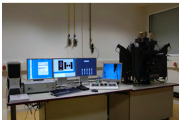
Fig. 28. Electron Microprobe (EMP) with five spectrometers at the CIC-UGR.
