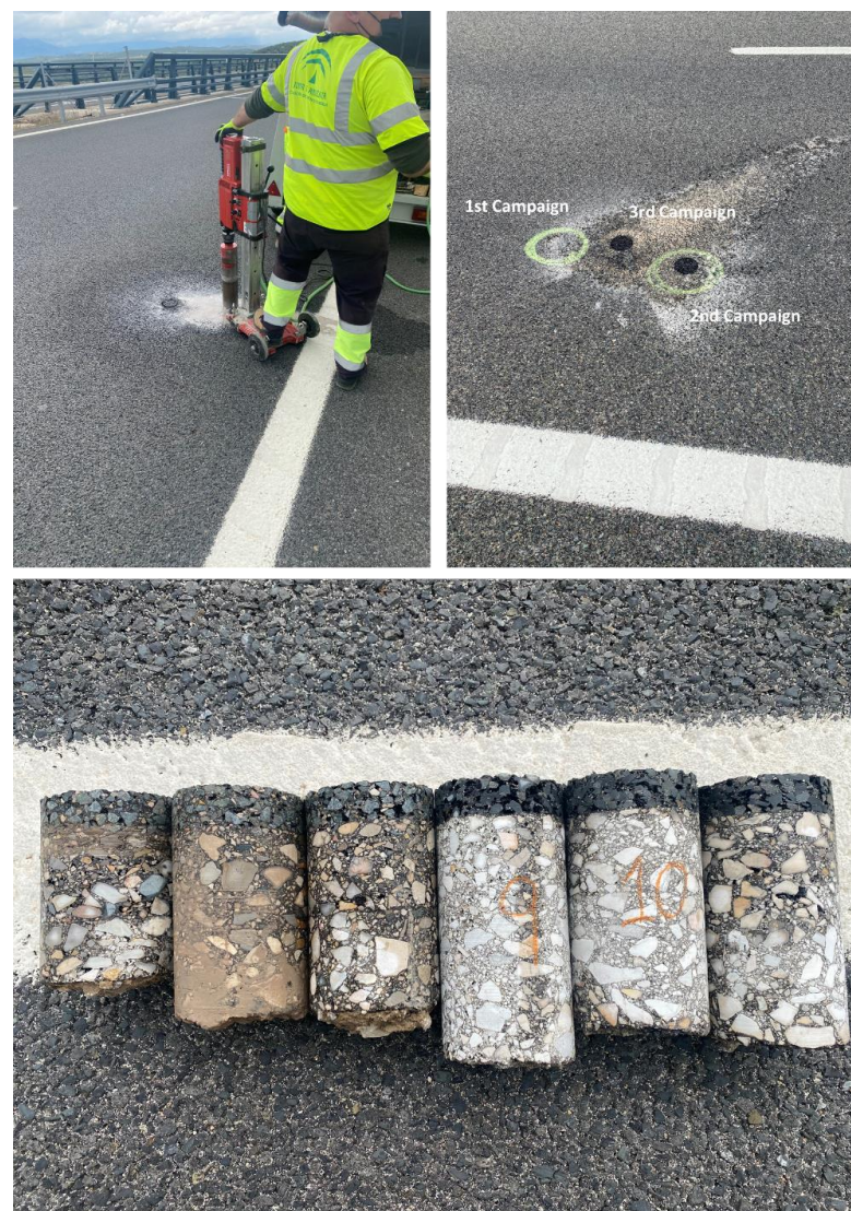
Figure 2. Details of the core extraction process.
