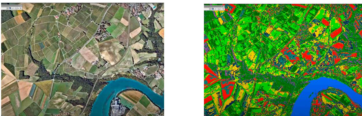
Figure 1. Classification of impervious surfaces using the SVM machine learning method (source: own elaboration based on orthophoto maps available on Geoportal— https://www.geoportal.gov.pl/ , accessed on 2 November 2022).
