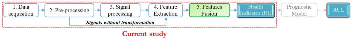
Fig. 3. Workflow of the present work as a part of the general steps in prognostics.
