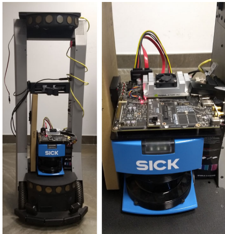
Fig. 1 PeopleBot robot equipped with LRF SICK LMS200 and a Jetson TX2 Developer Kit
