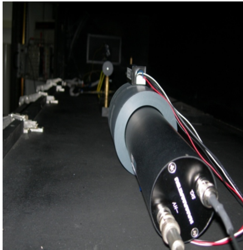
Figure 12. Photo-electron setup inside the dark box. In the foreground, the photo-electron PMT with the trigger PMT mounted on top it is seen. In the background, the LED pulser can be observed.
