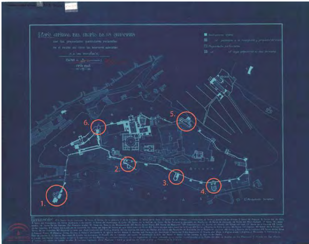
Figure 95: 1908, general plan of the Alhambra by Modesto Cendoya. All D-shaped bastions designed by Ramiro Lopez have been highlighted and numbered. 1. Torres Bermejas. 2. Justice Gate. 3. Gate of the Heads. 4. Seven Floors Gate. 5. Iron Bastion. 6. Tower of the Cube. © Archivo del Patronato de la Alhambra y el Generalife. 328
