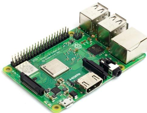
Figura 3.5: SBC Raspberry Pi 3B+
