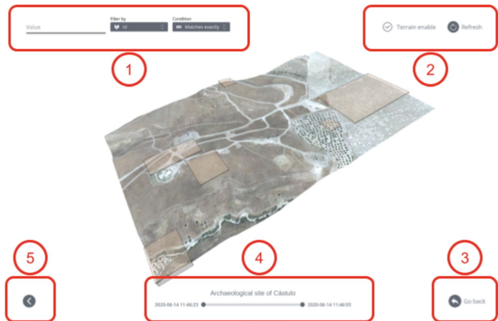
Fig. 7 Main screen of the application. (1) Attribute filtering options. (2) Switch for enabling/disabling the visualization of the digital elevation model of the terrain and refresh view control (to be used exceptionally, for example, if new data has been fed into the database while the current view is active). (3) Control to browse back in the data model. (4) Breadcrumb trail and time slider. (5) shows/hides a table with the data in the current view
