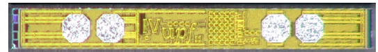
Figure 13. Picture of the ASIC, after sub-dicing, with the four bonding pads for external connections. Its final dimensions are approximately: 300 \mu\text{m} \times 2.5 \text{ mm} \times 204 \mu\text{m} .
