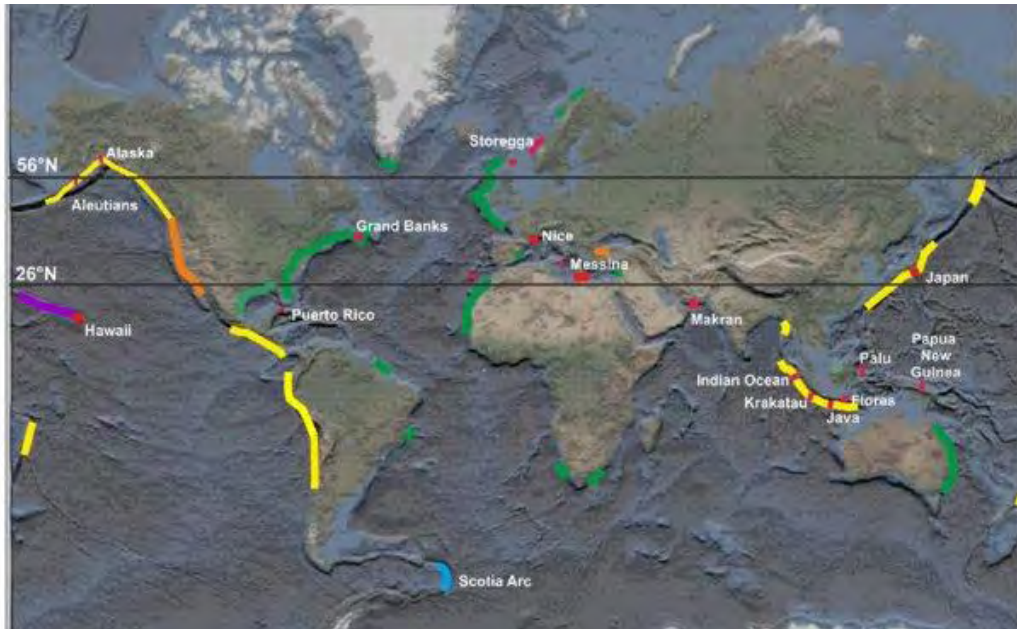
Figure 1-3. Global distribution of mapped submarine landslides (SLs): green, SLs on passive margins; yellow, SLs located along convergent margins; orange, SLs on strike-slip margins; purple, volcanoes; red, tsunamis associated with SLs. Submarine landslide tsunamis (in red) are mainly located along convergent margins, but also along passive and strike-slip margins and on flanks of volcanoes (Sassa et al., 2022).
