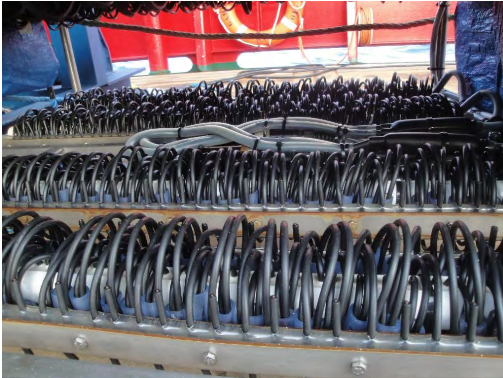
Figure 3-7. Image showing an example of sparker system with several electrodes.
