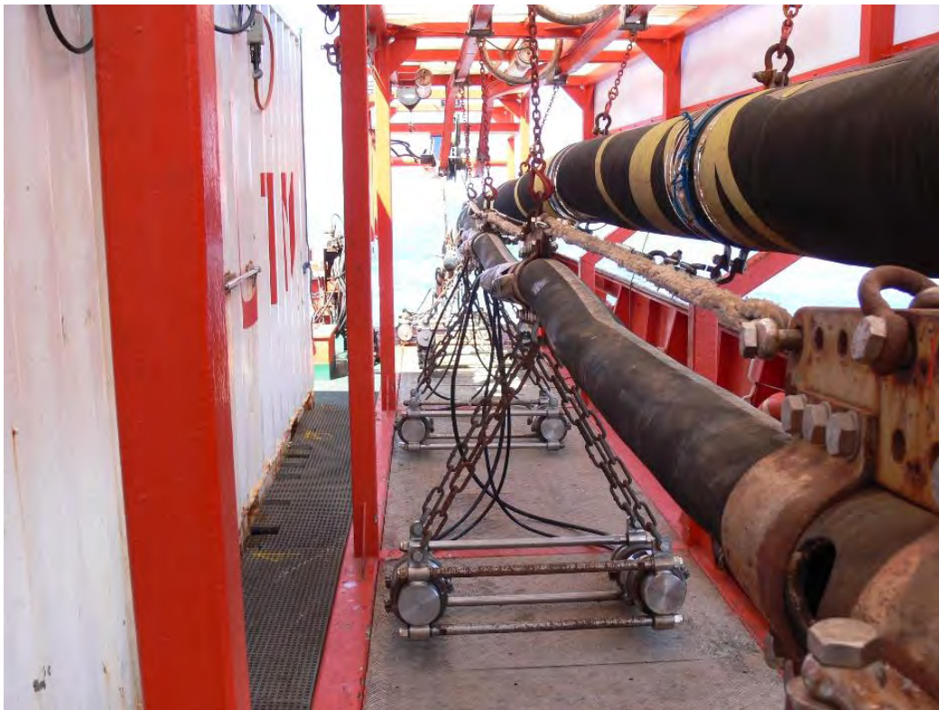
Figure 3-6. Airgun seismic array with 8 guns.
