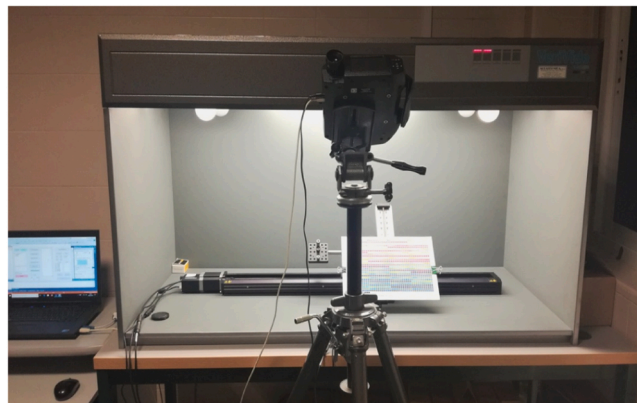
Fig. 1. Experimental set-up for obtaining the color gamuts. Automated displacement modules were used inside the light cabinet; a spectroradiometer, sample pattern, and computer used for these measurements.
