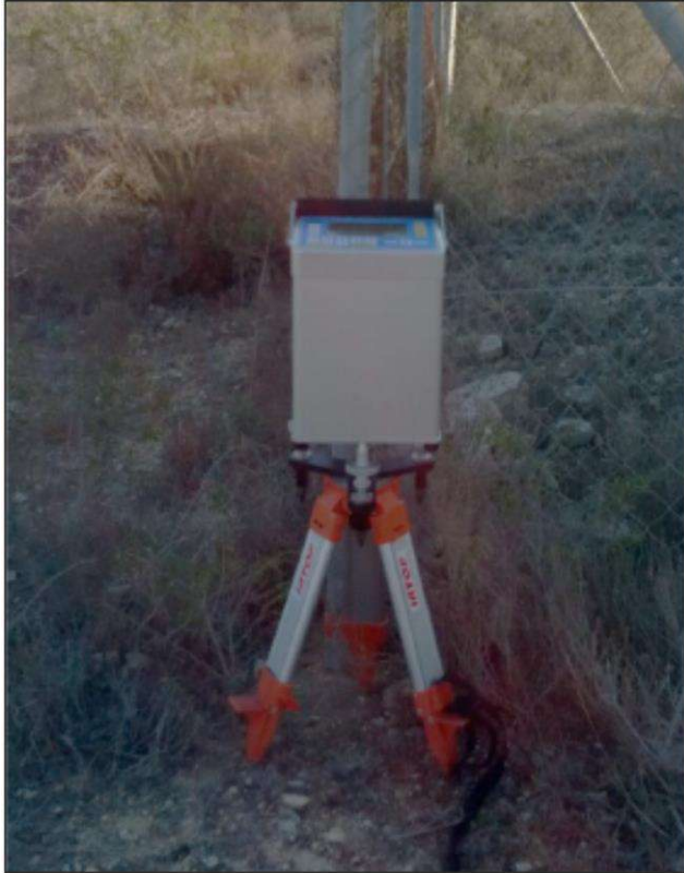
Figure 3.1. Gravimeter Scintrex CG-5 Autograv with tripod used to acquire gravity data during this Ph.D. Thesis.
