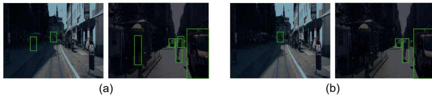
Figure 7.8: Target detection in night frame with (a) sensor fusion algorithm and (b) only camera.
