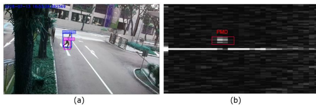
Figure 6.7: (a) Image extracted from the Object detector using the camera data. (b) Result of the sensor fusion approach proposed in this paper.
