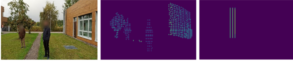
Figure 8.1: From left to right: original environment camera image, LiDAR depth map and radar depth map.
