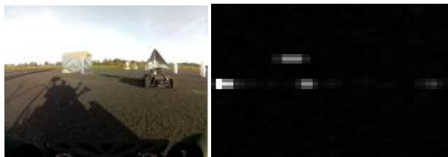
Figure 6.8: Camera and radar range Doppler map image from the second dataset.
