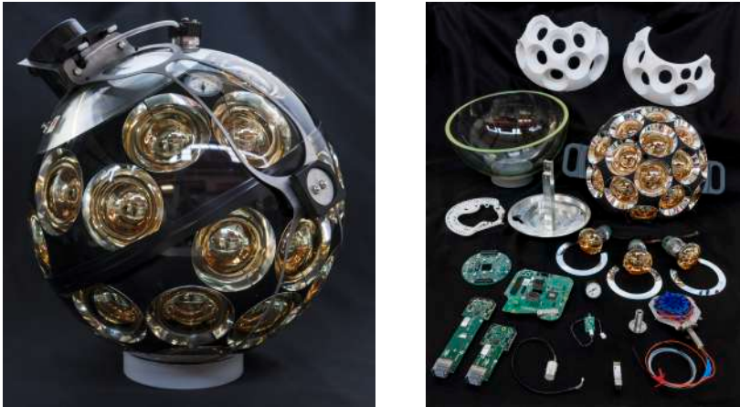
Figure 4.4: A KM3NeT Digital Optical Module (left) and its components (right). From [182].
