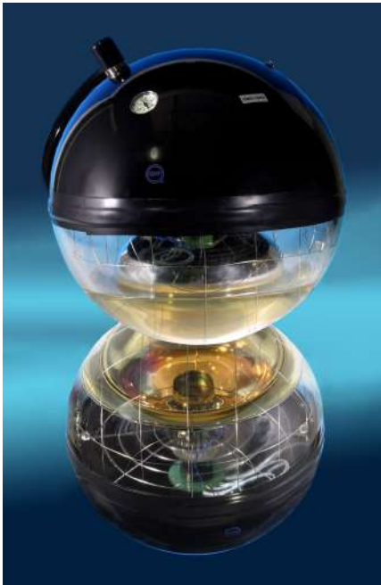
Figure 2.3: A photograph of an ANATRES optical module positioned on a mirror (left) and an schematic drawing of an storey with 3 OMs pointing downwards. From [98, 104].
