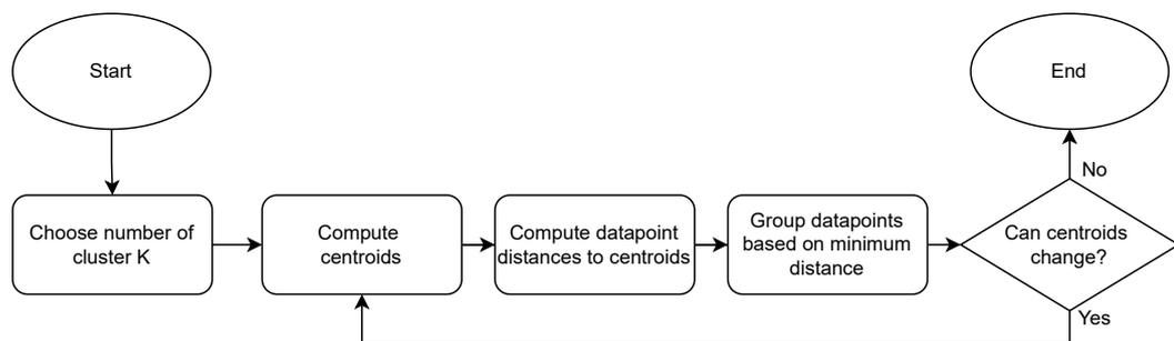
Fig. 5.2.: Flow diagram of the K-Means algorithm.
