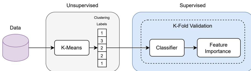
Fig. 5.3.: Feature importance analysis of clustering results with a supervised approach.
