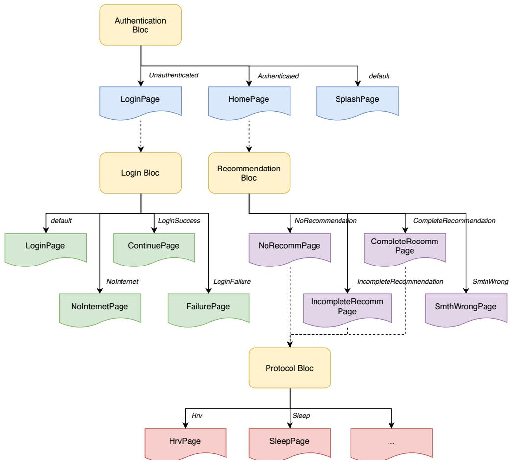
**Fig. 3.4.:** Bloc–state–UI structure of the ATOPE+ app. Blocs connect with UI (pages or views) through states.
