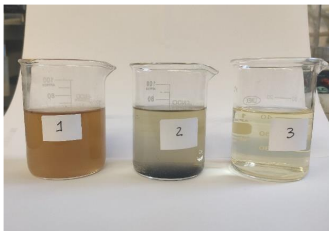
Fig. C.10 (1) Ten-fold diluted OMW, (2) OMW after CWPO (240 min) with OSAC-Fe-IWI deposited, and (3) OMW after CWPO without catalyst.
