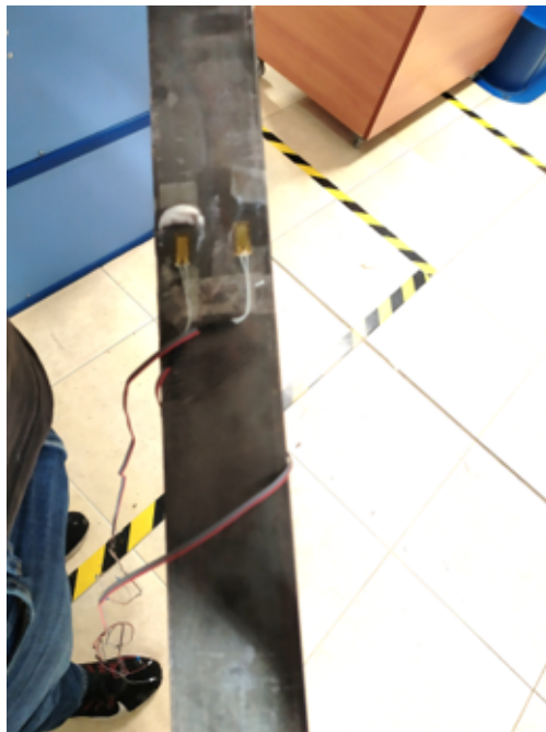
Figure 5.13 – Steel plate with strain gauge glued
