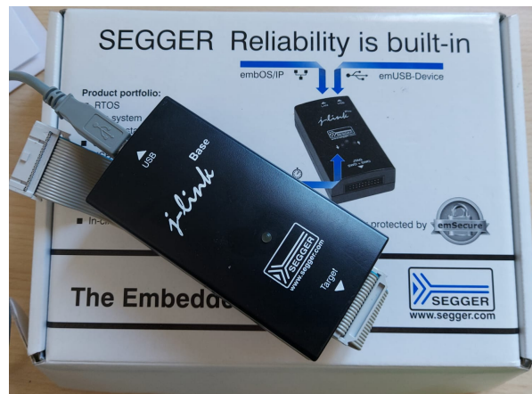
Figure D.1 – J-Link Device from SEGGER [54]
