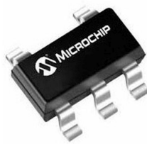
Figure 2.22 – Li-Polymer Charge Management Controller Module [19]
