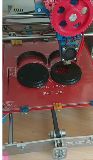
Video 5.2 – 3D printer fabricating the "can" (double click in Adobe Acrobat)
