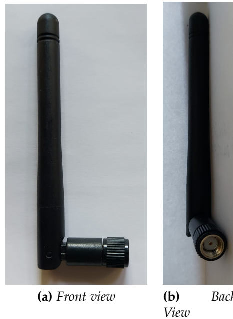
Figure 4.41 – 433 MHz SMA antenna module [30]
