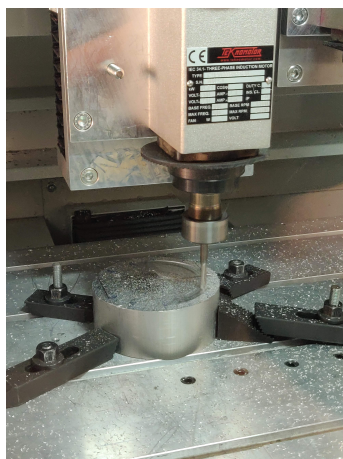
(a) Semisphere Milling
