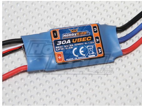
Figure 3.27 – ESC 30A Driver [17]
