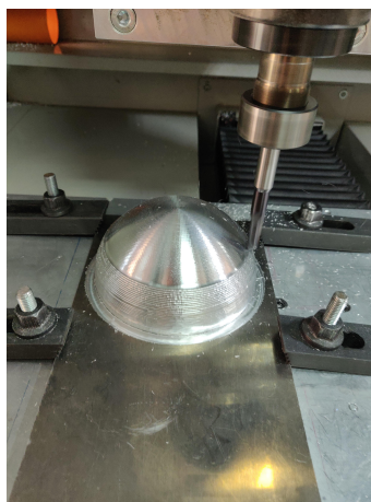
(b) Defining Semisphere Circular Profile
