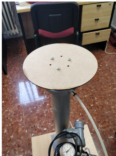
Figure 4.4 – Wooden Platform for SP
