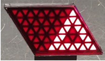
Fig. 13. Digital QD-LED device designed in this work with dynamic lighting scenario example (hazard warning mode). Car-to-X communication in rear-lamps [7], [8].
