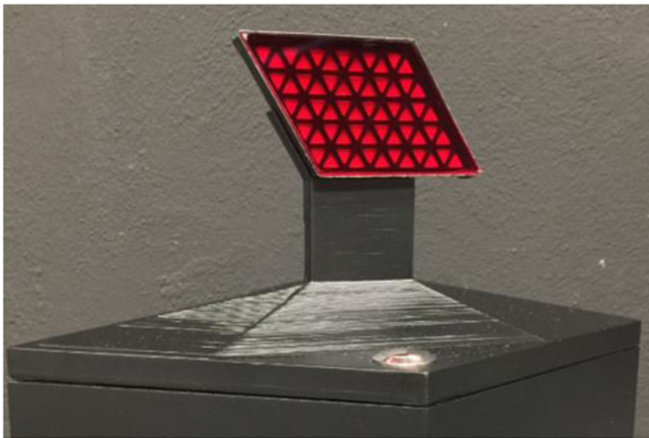
Fig. 4. Dynamic photoluminescence QD-LED application for automotive lighting systems. Designed for this work.
