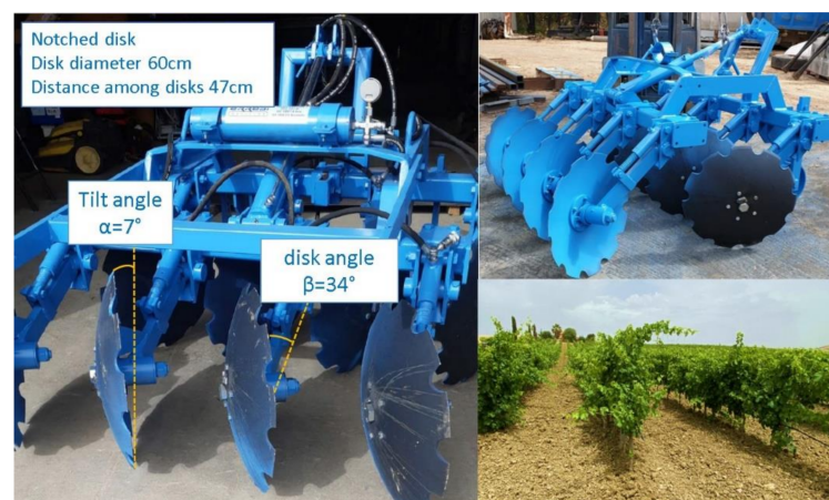
Figure 1. Standard disk plough used during the tillage tests: tilt angle ( \alpha ) between the disk plane and the perpendicular to the field plane; disk angle ( \beta ) between the disk plane and the travel direction.
