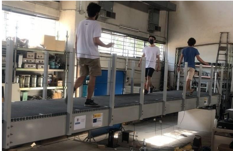
Figure 2. Dynamic test: three pedestrians walking.
