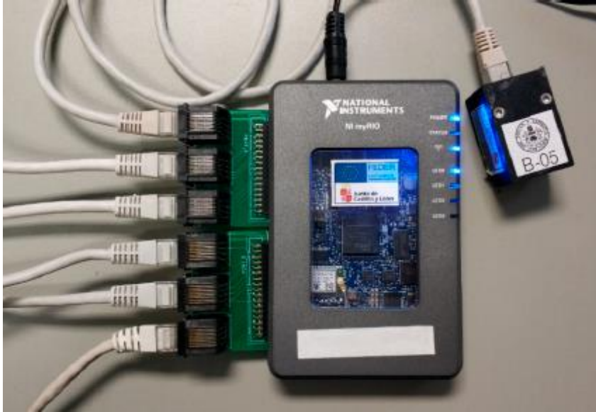
Figure 3. MyRIO device with two adapter boards and an accelerometer.
