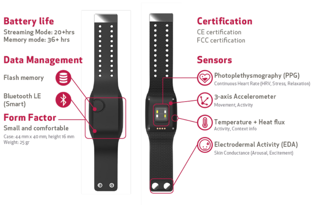
Fig. 2.22 E4 wristband for real-time physiological data streaming and visualisation proposed by empatica [73].
