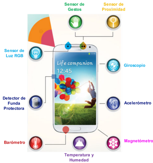
Fig. 2.24 Mobile device that stands out because it integrates environmental temperature and humidity sensors in addition to the conventional ones [171].
