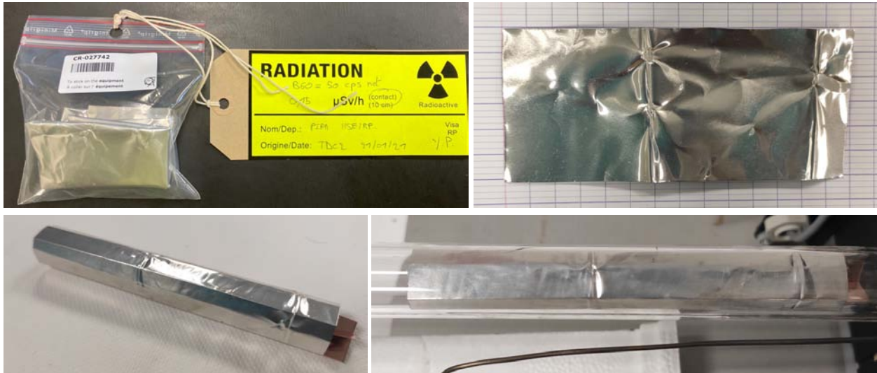
Figure 6.8: Activated Al foil from TDC2 (upper left), portion to be used to create the sample (upper right), sample ready to be used (lower left) and sample inside the quartz tube (lower right).
