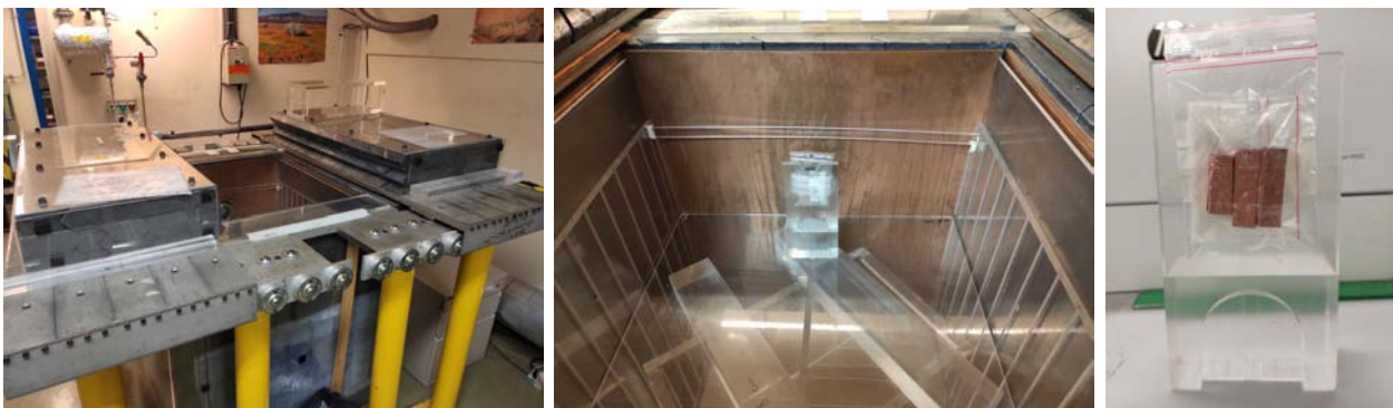
Figure 6.1: Pictures of the setup used in the gamma-ray spectrometry laboratory in building 24. GE5-B10162 detector open (left), interior of the detector with one of our radioactive samples placed and ready to be measured (centre) and detail of the samples and the support, used for an optimum alignment of the samples and the detector (right).
