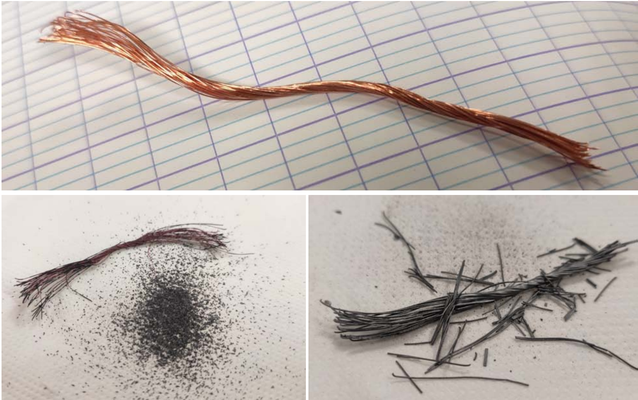
Figure 6.14: Cu filaments at 800 °C and 1000 °C in an air atmosphere. Filaments before heating (upper picture). Filaments after 20 min at 800 °C; the powder next to them came off after a brief manipulation (lower left). New filaments after 20 min at 1000 °C, they became easily breakable (lower right).
