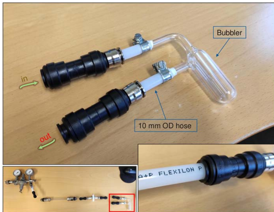
Figure 6.5: Detail of the bubbler used to monitor the gas flux. Similarly to the HEPA filter, a 10 mm hose plus connections was used to guarantee tight joints.
