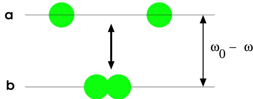
**Figure 1.** Schematic representation of the model used in this work for the atom–diatomic coexistence. This is a two-level model. Diatomic molecules (b) are in the lower level, while single atoms (a) are in the upper level. The quantity  $\omega_0 - \omega$  represents the energy needed for separating the molecule into its two single atoms. This figure was taken from [16].
