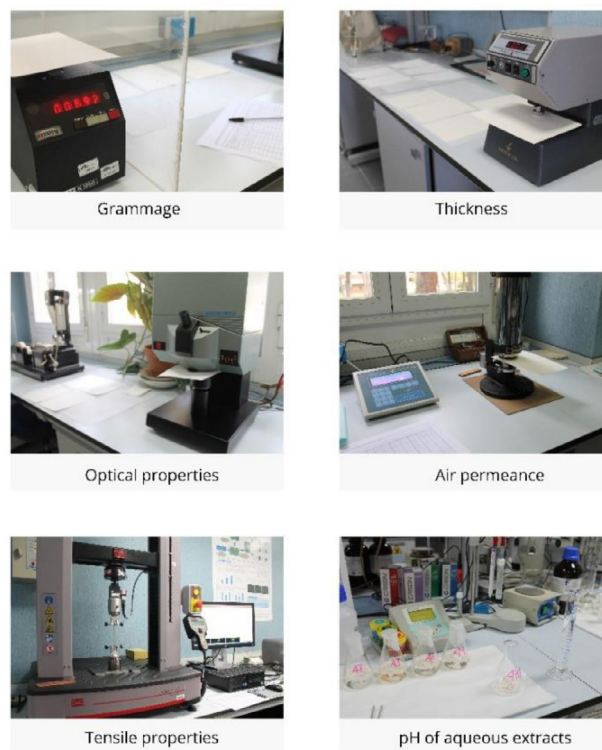
Fig. 3. Photographs of the different actions to characterise the physico-chemical, mechanical and optical features of the paper samples subsequent to the two bleaching (ALR and H_2O_2 ) treatments.
