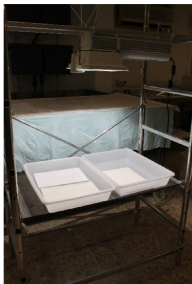
Fig. 2. View of the technique of paper bleaching by means of controlled artificial light radiation (ALR).
