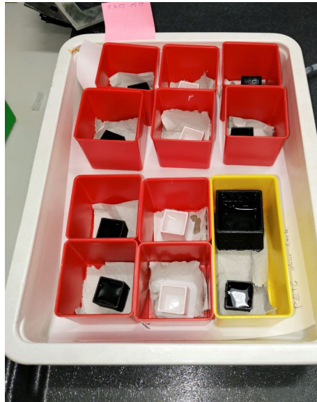
Figure 6.12: Test setup for verifying the liquid- and alkali-tightness of different filament and varnish combinations.
