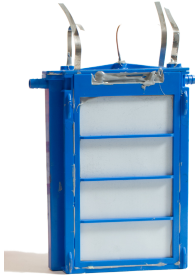
Figure 2.13: Photo of the zinc-air cell under development.
