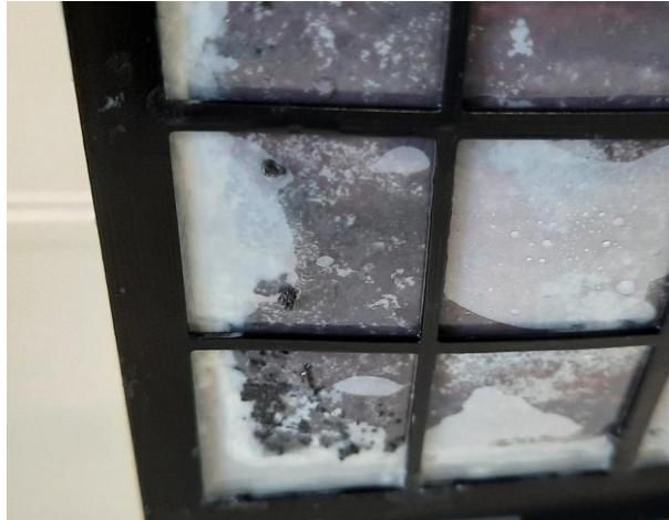
Figure 5.15: Zinc dendrites penetrating the separator.
