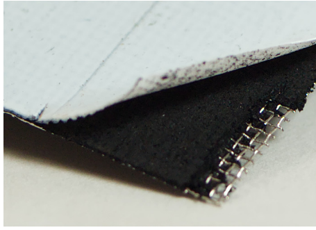
Figure 2.10: Structure of zinc-air gas diffusion electrode.
