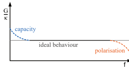
Figure 6.10: Characteristics of the ratio of the measurement conductivity and the actual conductivity depending on the modulation frequency.
