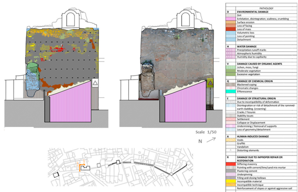
Figure 9. Elevation of pathologies of the Gate of Hernán Román. Source: PREFORTI Project. I. Bestué Cardiel.
