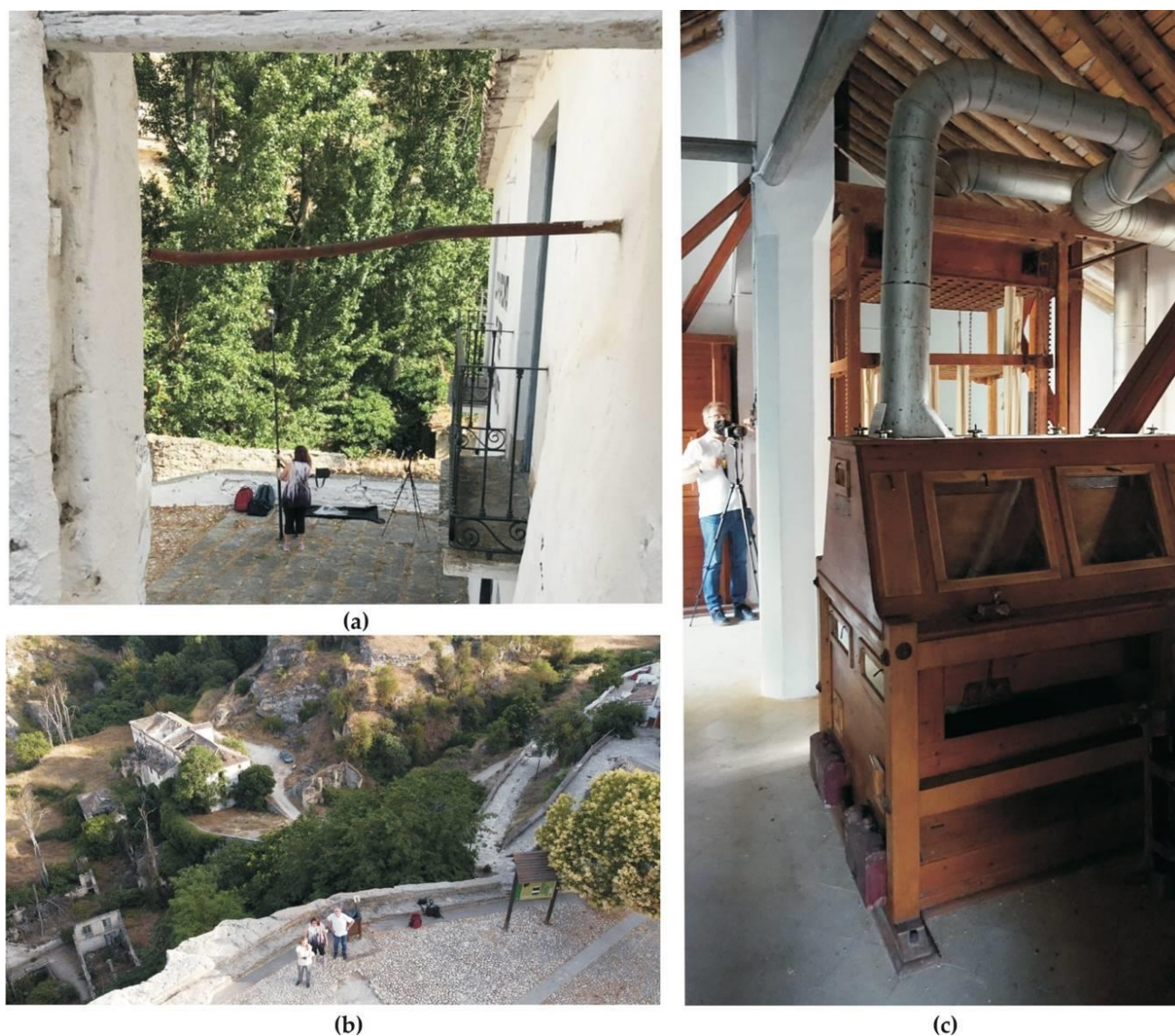
Figure 6. Photographs of the field work for the photographic and photogrammetric record: (a) photographic equipment and pole (J.G.M.-S., M.d.C.V.-L. and C.R.-M.); (b) image taken with DJI Mini 2 Drone (M.d.C.V.-L.); (c) Nikon D90 camera and tripod inside the Fábrica de Harinas la Purísima (J.G.M.-S.).
