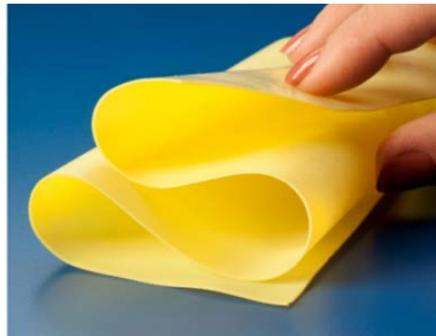
*Figura 8. Aerogel flexible de poliimida. Nota: Adaptado de “Biopolymer Aerogels and Foams: Overview and Outlook for Future Space and Terrestrial Applications at NASA.” Viggiano, R., NASA Glenn Research Center. <https://ntrs.nasa.gov/api/citations/20180005488/downloads/20180005488.pdf>*
