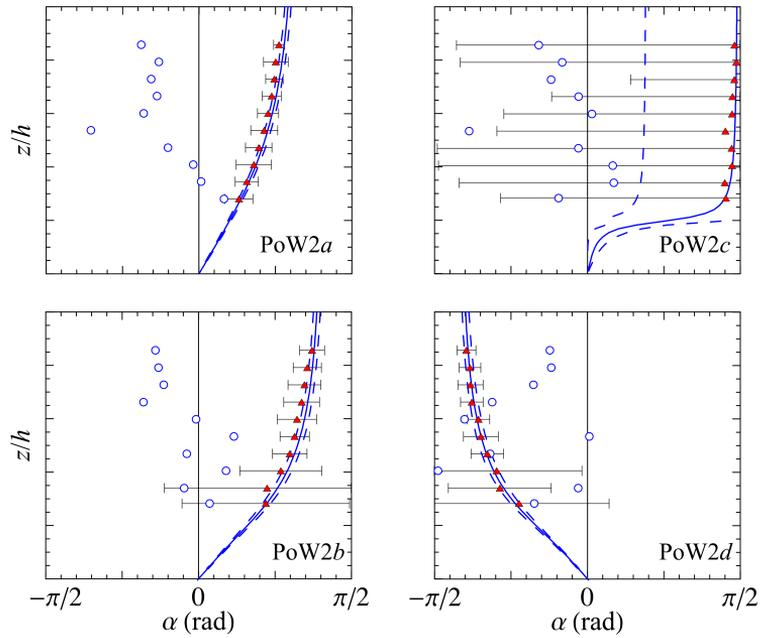
Figure 4.29: Experiments P2a–d, paddle waves with opposing wind (same reflection, different LDV positions). Wave and turbulent principal angles  $\tilde{\alpha}_p$  and  $\alpha'_{exp}$ , respectively. Triangles and circles are periodic and fluctuating experiments, respectively, while solid lines are theoretical values. Error bars are two standard deviations, dashed lines are confidence intervals to 95% level.
