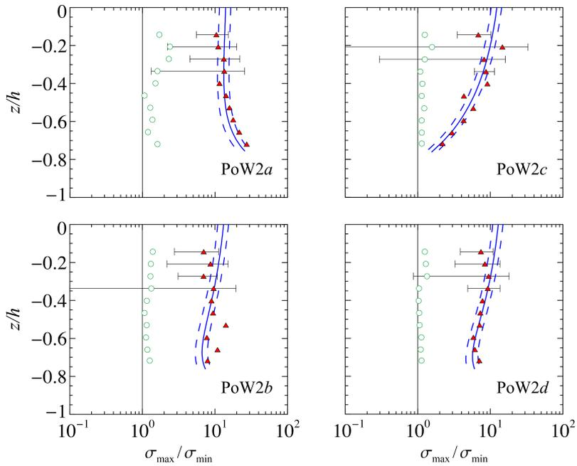
Figure 4.27: Experiments PoW2a–d, paddle waves with opposing wind (same reflective conditions, different LDV sections). Ratio of the maximum to minimum principal stress  $\sigma_{\max}/\sigma_{\min}$ . Triangles and circles are experimental values for periodic and fluctuating components, respectively, with error bars equal to one standard deviation. Solid lines are theoretical values from equation (1.27), while dashed lines are confidence intervals to 95%.
