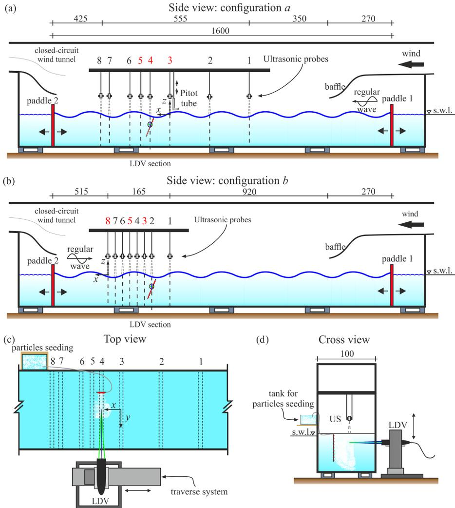
Figure 2.1: (a) Side view of the experimental set-up for larger US spacings (configuration *a*). (b) Side view of the experimental set-up for narrow US spacings (configuration *b*). (c) Top view of the flume (configuration *a*). (d) Cross view of the flume. No wind blockage was observed in proximity of paddle 2, indicating good performances of the closed-circuit wind tunnel.
