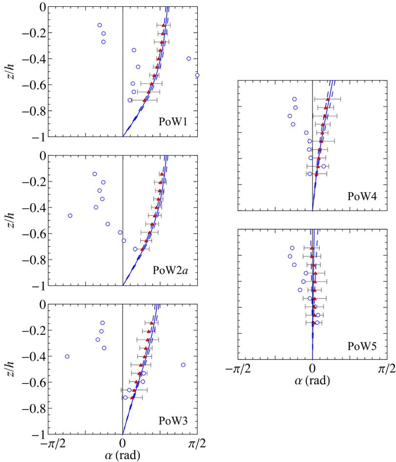
Figure 4.28: Experiments PoW1–5, paddle waves with opposing wind (different reflection, same LDV section). Wave and turbulent principal angles  $\tilde{\alpha}_p$  and  $\alpha'_{exp}$ , respectively. Triangles and circles are periodic and fluctuating experiments, respectively, while solid lines are theoretical values. Error bars are two standard deviations, dashed lines are confidence intervals to 95% level.
