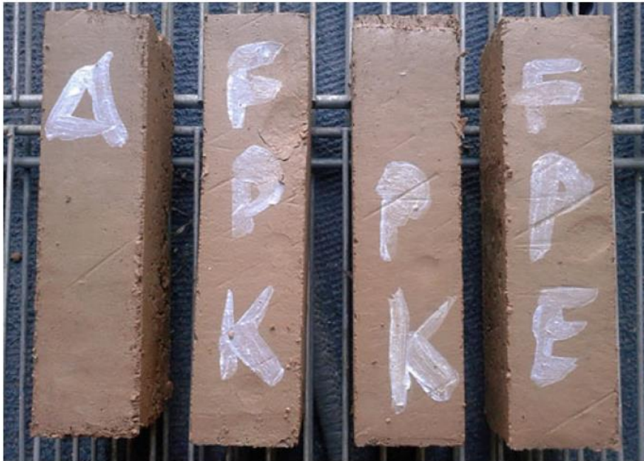
Fig. 6 Earth mortar specimens kneaded with water or plant infusions
