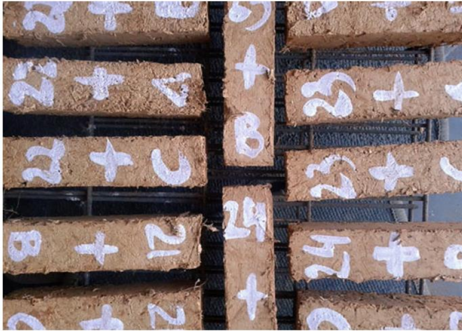
Fig. 7 Lime stabilized hemp-clay concrete test specimens
