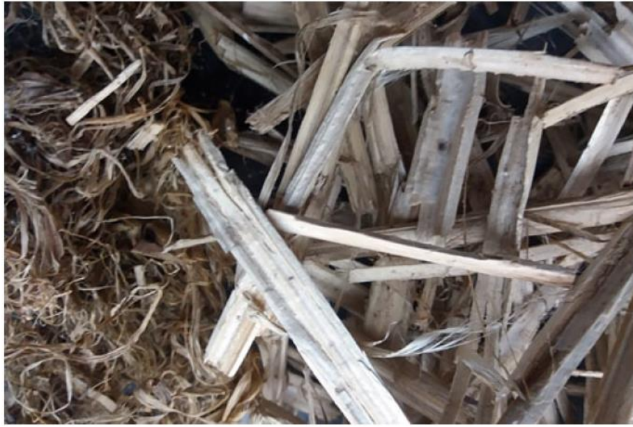
Fig. 4 Moroccan hemp core and fiber after 14 days of submersion in water and drying
