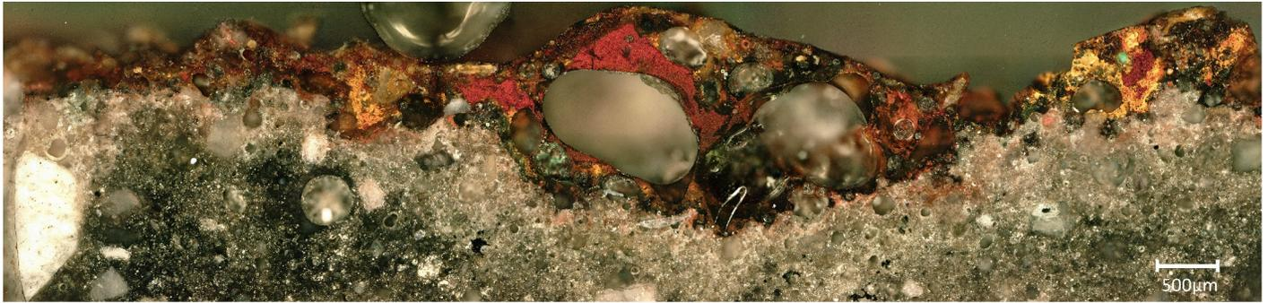
**Fig 5. XPL micrograph of G11 with the thickest of all slag layers analysed.** Note the interaction between the slag layer and the ceramic and the development of bloating pores. (Scale = 500 $\mu$ m).
