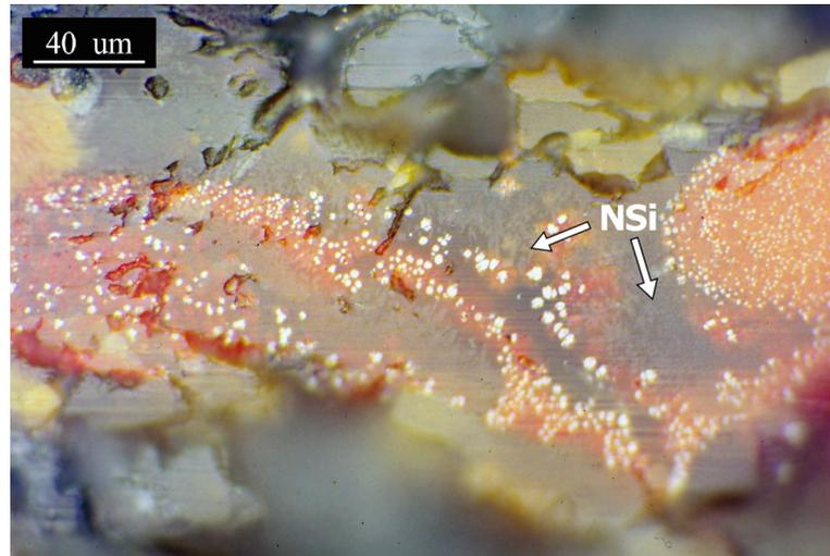
**Fig 13.** PPL micrograph of PA6325 showing whitish prills of cuprite, its reddish exsolution and small neosilicates (NSi, light grey) in the darker grey matrix. (Scale = 40µm).
