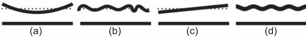
Figure 4. Typical defects of Fabry–Pérot etalons: (a) spherically shaped with a peak-to-peak excursion \Delta s_s ; (b) irregularities following a Gaussian distribution with a variance \Delta s_g^2 ; (c) linear wedge with a peak-to-peak deviation \Delta s_p ; and (d) sinusoidal defect of peak-to-peak amplitude \Delta s_a .
