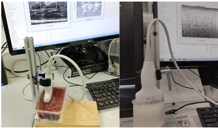
Figure 3.3: Set-up for measurements using SWEI. The picture was taken during the measurements at the Ultrasonics Lab at the University of Granada. In the left image, the ex vivo liver sample is measured while one of the hydrogel phantoms is shown in the right image. Adapted from [2].
