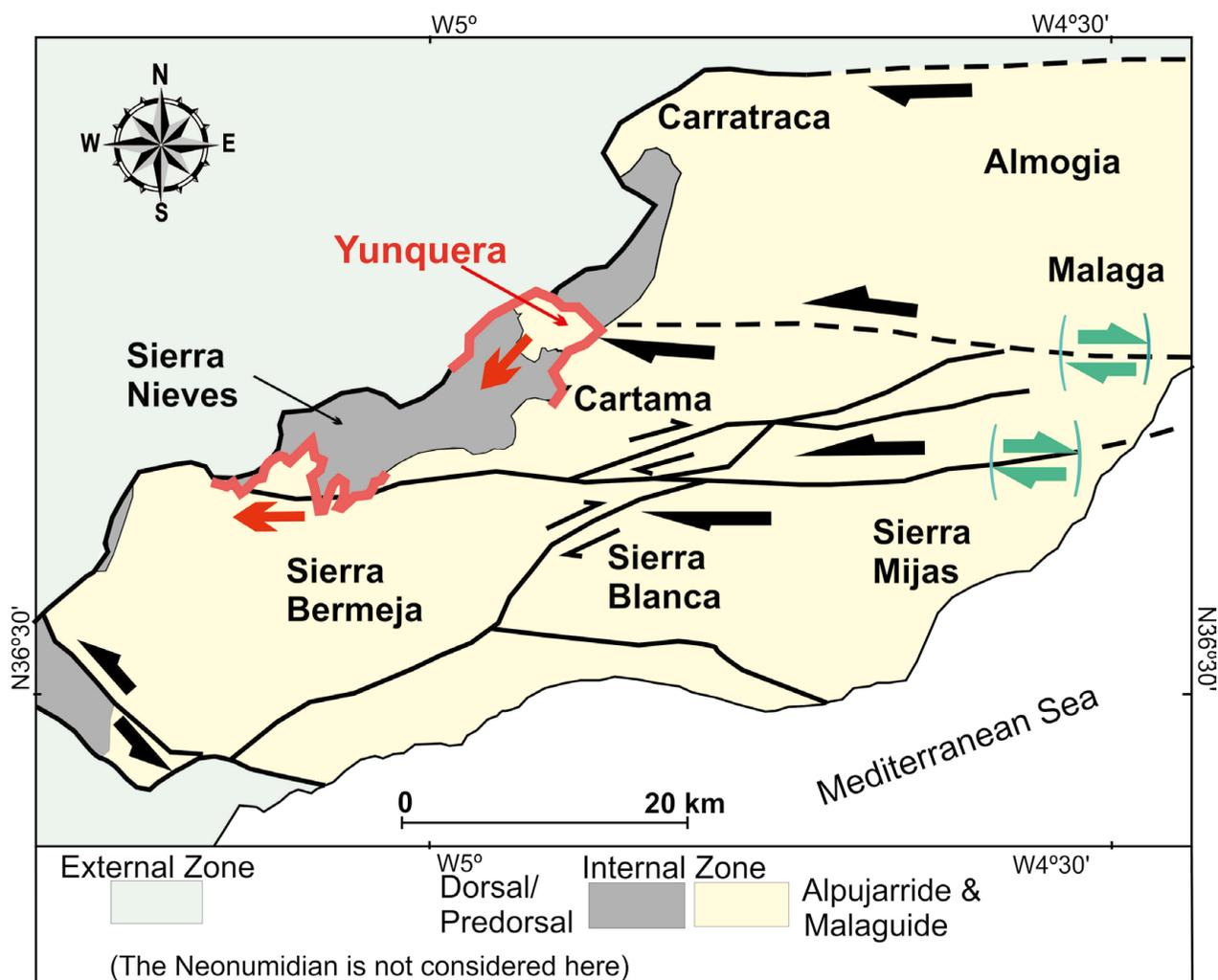
Figure 9.— Tectonic scheme in which the oblique cuts (in red) underwent by the Dorsal in the Yunquera area and to the south of the Sierra de las Nieves are indicated. The red arrows indicate the local directions of displacements. In green, the relative displacements of the fault blocks are marked.
