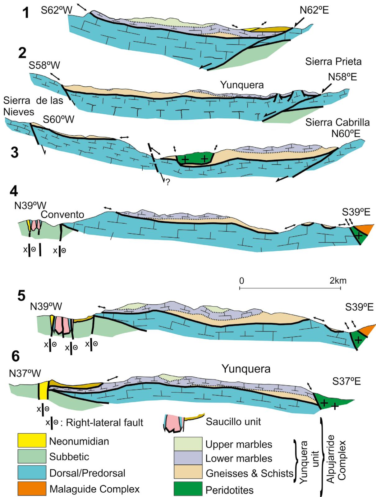
Figure 7.— Geologic cross sections of the study area. Their positions are indicated in figure 6. The symbol (x/o) indicates dextral strike slip faults.
