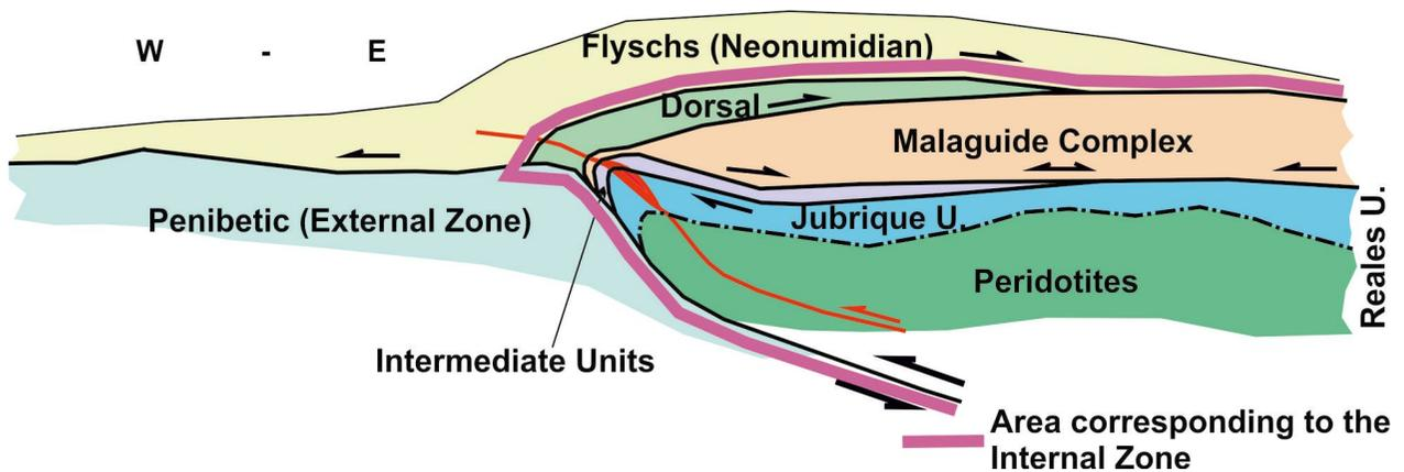
Figure 4.— Interpretation of the general structure of the Western Betic Internal Zone. The red line tries to indicate the approximate position of the immediately later thrust forming the Yunquera unit (red area).
