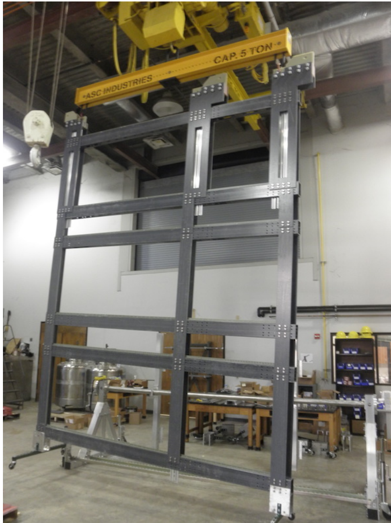
Figure 3.25. Top and center endwall FC module frames hanging.
