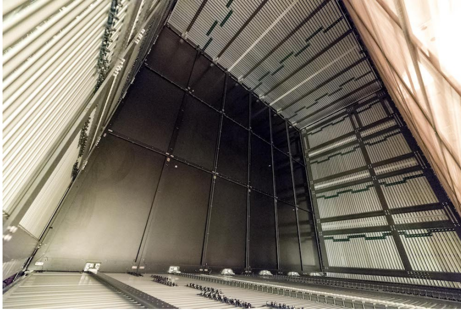
Figure 3.18. One of the two drift volumes of ProtoDUNE-SP. The FC modules shown enclose the drift volume between the CPA array (at the center of the image) and the APA array (upper right). The endwall FCs are oriented vertically; the top and bottom units are horizontal. The staggered printed circuit boards connecting the endwall FC profiles are the voltage divider boards.
