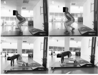
**Figure 1.** Evaluation of maximal isometric forces. Isometric squat with knee flexion at 90° (A), isometric squat with dominant knee forward and flexed at 90° (B), maximal isometric force of the lower-body exerted on starting blocks with dominant knee forward and flexed at 90° (C), maximal isometric force of the lower-body exerted on starting blocks with both knees at 90° (D).
