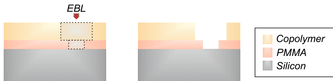
Figure 5.3. PMMA-Copolymer profile after EBL exposure. A thinner sidewall profile is obtained with a polymer-copolymer configuration.
