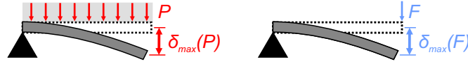
Figure 4.26. Representation of an applied pressure or force on a cantilever. Schematic (left) of cantilever loaded with a uniform pressure, P , and a cantilever loaded with a force, F , at one end.
