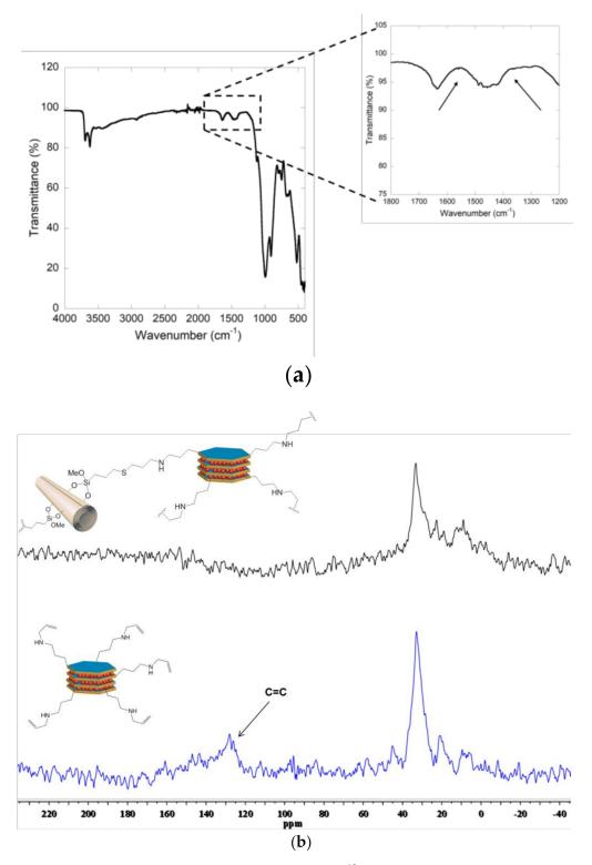
**Figure 2.** (a) FTIR spectrum of HNTs-Ht nanomaterial; (b) solid state <sup>13</sup>C NMR spectra of Ht-Allyl (blue line) and Hal-Ht (black line) nanomaterials.
