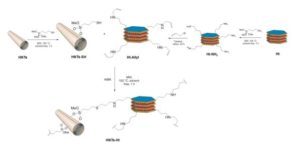
Scheme 1. Schematic representation of HNTs-Ht nanomaterial synthesis.
