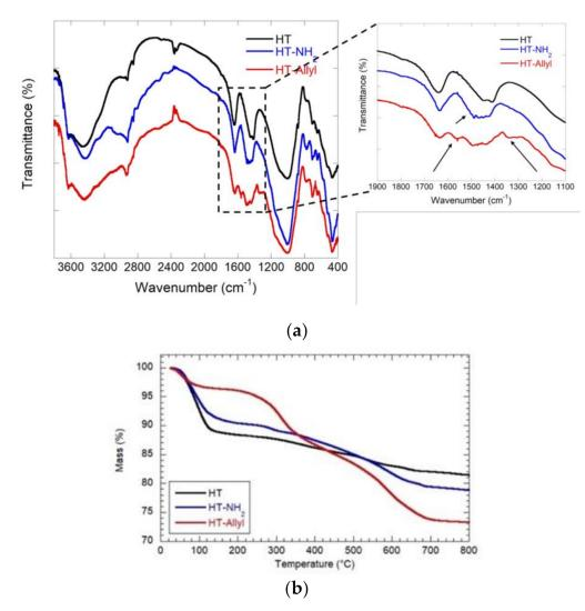
Figure 1. (a) FTIR spectra of pristine Ht, Ht-NH<sub>2</sub> and Ht-Allyl; and TG curves (b) for pristine Ht, Ht-NH<sub>2</sub> and Ht-Allyl.
