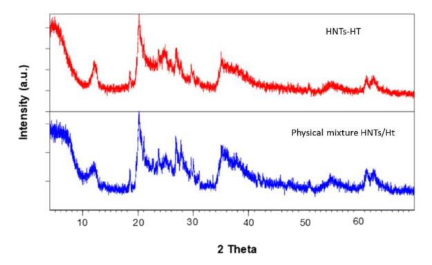
Figure 4. Comparison between the XRD patterns of HNTs/Ht physical mixture and HNTs-Ht nanomaterial.
