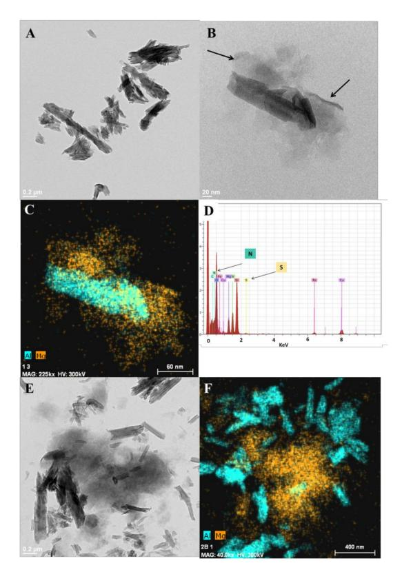
**Figure 3.** (**a**,**b**) TEM image of HNTs-Ht nanomaterial (scale bar 200 and 20 nm, respectively); (**c**) corresponding EDX image of Al and Mg from STEM image (scale bar 60 nm); (**d**) EDX spectrum of the HNTs-Ht nanomaterial; (**e**) TEM image of the physical mixture constituted by HNTs and Ht (scale bar 0.2 µm); and (**f**) the corresponding EDX image of Al and Mg from STEM image (scale bar 0.4 µm).
