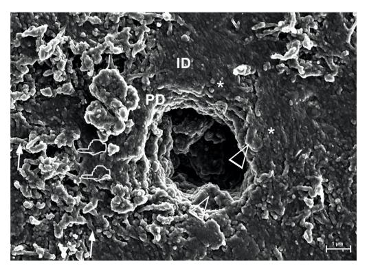
**Figure S1.** Field emission scanning electron microscopy (FESEM) image of a dentin surface. Peritubular dentin (PD) and intertubular dentin (ID) are clearly differentiated. Some collagen fibers were demineralized (pointers) or appeared mineralized (arrows). Mineralized clusters perform partially covering both the PD and the ID (arrow heads). A single layer of minerals partially shielded the ID and some extension of the PD (asterisks).
