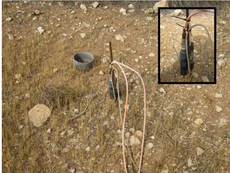
Figure 11. Shallow \text{CO}_2 and temperature sensors. Photos from Amoladeras experimental site.
