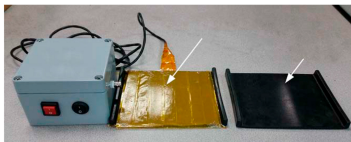
Figure 9. Signal conditioner, rail pad sensor and rail pad [49].
