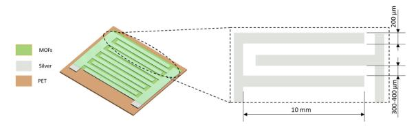
Figure 1. Schematic image of the fabricated sensor and detailed dimensions of the IDE.
