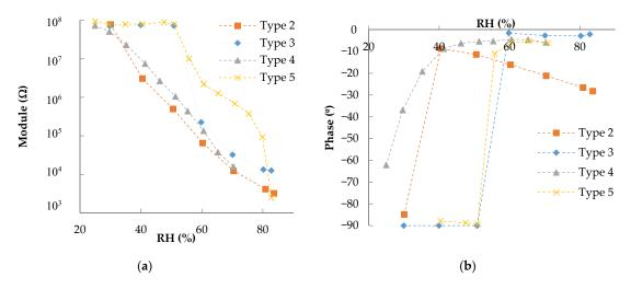
**Figure 3.** Impedance response towards RH at 100 Hz and 40 °C for the different deposited layers with distance between consecutive fingers of 300  $\mu$ m: (**a**) module and (**b**) phase.
