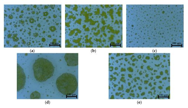
**Figure 2.** Optical microscope images for the spray coating with the different fabrication parameters: type 1 (**a**); type 2 (**b**); type 3 (**c**); type 4 (**d**); type 5 (**e**).
