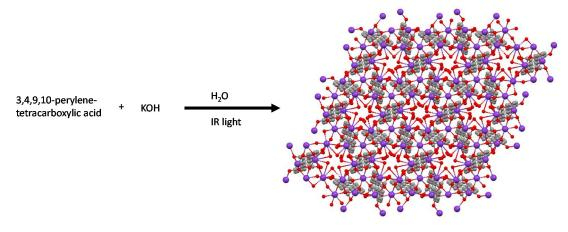
Figure A3. Synthetic scheme with the structure of the MOF.
