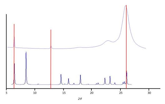
**Figure A4.** Top: Experimental PXRD of sample after spray coating deposition. Down: Theoretical PXRD obtaining of single crystal data.
