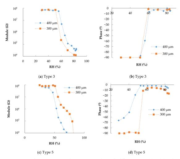
**Figure 4.** Impedance response towards RH at 100 Hz and 40 °C for different spacing: (**a**) module and (**b**) phase for type 3; (**c**) module and (**d**) phase for type 5.
