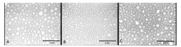
**Figure 3.** Microscopic scale bidimensional image of foams formed by (**A**) 3% POL, (**B**) 3% POL + 0.3% HA, and (**C**) 3% POL + 0.1 mM F68. Foam samples were produced with the double syringe method standardized protocol (1:4 liquid/air, 50 cycles, 0.9% NaCl, and 20 °C), and the images were taken after 1 min.
