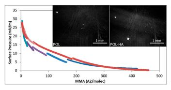
**Figure 6.** Surface pressure ( $\pi$ )-mean molecular area (MMA) isotherm of POL monolayers in pure water subphase (blue and purple) and in HA 3 × 10<sup>-3</sup> (g/L) subphase (red and pink). MicroBAM images of POL and POL + HA at  $\pi$  = (12 ± 1) mN/m.
