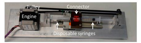
**Figure 1.** In house double syringe method used for foam designed at the University of Granada and manufactured by Producciones Científicas y Técnicas S.L. (Gójar, Spain).
