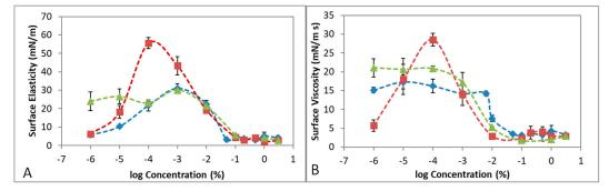
**Figure 5.** (A) Surface dilatational elasticity (1 Hz). (B) Surface dilatational viscosity (0.01Hz) attained after 1 h of adsorption at constant surface area, 0,9% NaCl and T = 20 °C as a function of bulk concentration of POL. POL (blue rhombus), POL + 0.3% HA (red squares), and POL + 0.1 mM F68 (green triangles). Values plotted are mean values of three independent measurements, and standard deviations are plotted as error bars. Lines are a guide for the eye.
