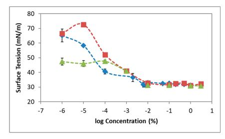
**Figure 4.** Surface tension values after 1 h of adsorption at constant surface area, 0.9% NaCl and T = 20 °C as a function of bulk concentration of POL. POL (blue rhombus), POL + 0.3% HA (red squares), and POL + 0.1 mM F68 (green triangles). Values plotted are mean values of three independent measurements, and standard deviations are plotted as error bars. Detailed statistical analysis of data is shown in Figure S3. Lines are a guide for the eye.
