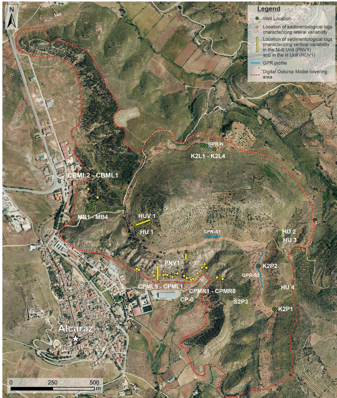
Fig. 3.17. Satellite image of the study area showing the location of the wells, sedimentological logs and GPR profiles. In addition, the area incorporated into the digital outcrop model is also shown. Acronyms correspond to the names attributed to the sedimentological logs, well data and/or GPR profiles.
