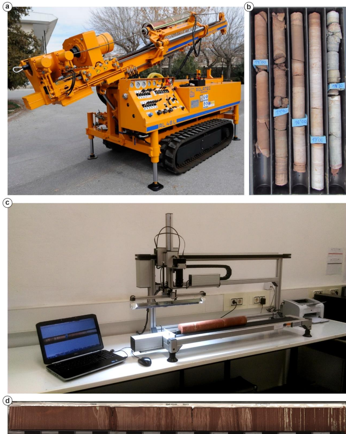
Fig. 3.8. (a) CIC Rolatec RL-48 rotary drill used in this study. (b) Example of recovered cores. (c) CIC core scanner Smartcube CIS 1000L used in this study. (d) Example of core tray displaying 1m of slabbed core.
