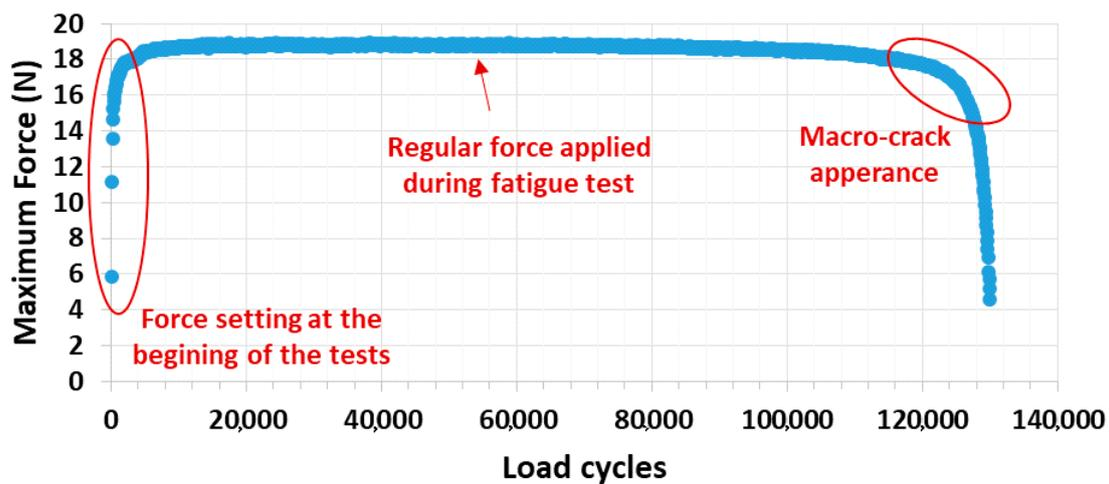
**Figure 6.** Example of the maximum force vs. load cycles graph obtained from the fatigue 3-point bending test in the DMA.
