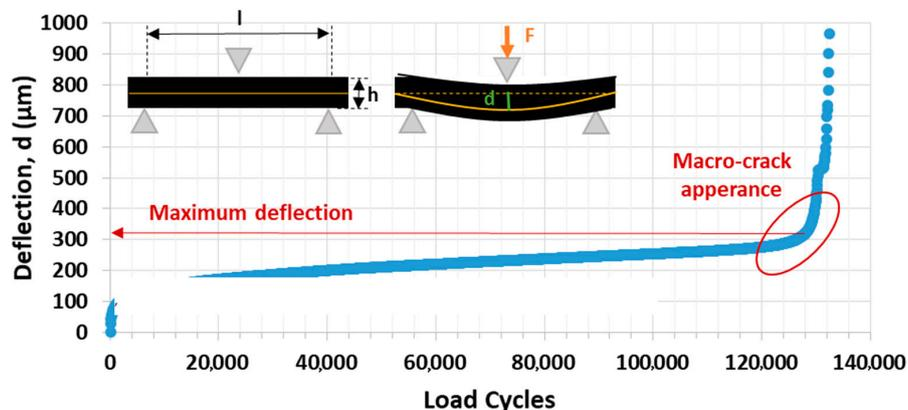
**Figure 7.** Deflection  $d$  ( $\mu\text{m}$ ) registered during the 3-point bending fatigue tests.
