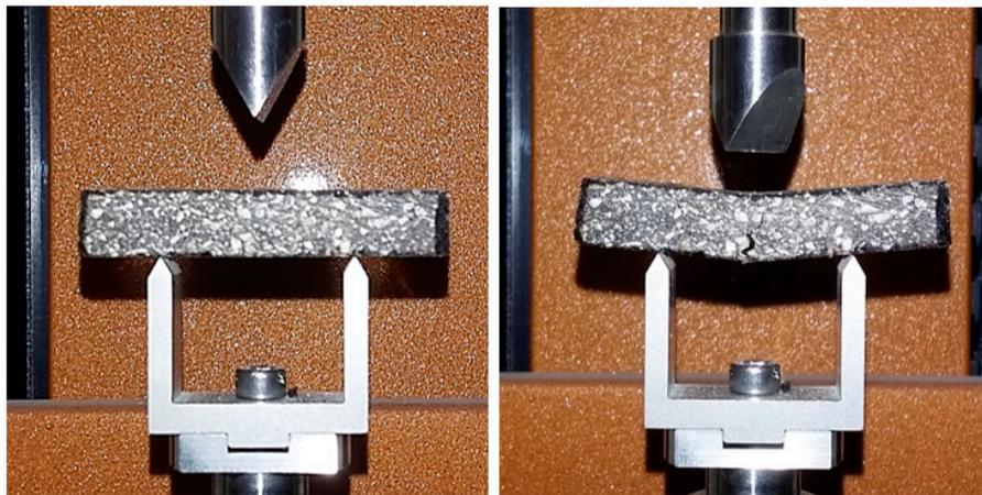
Figure 4. Aspect of the mortar specimen before and after fatigue with the 3-point bending test in the DMA.
