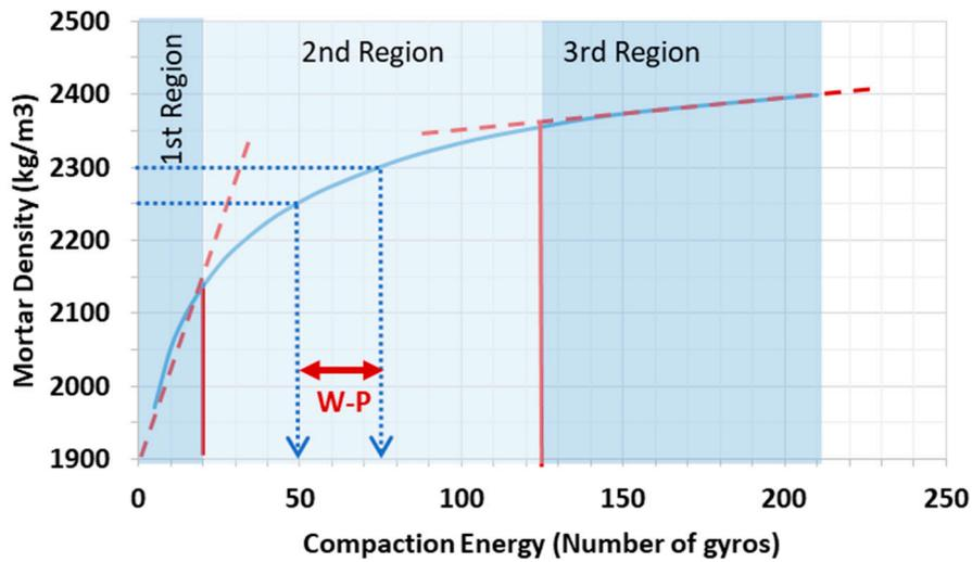
Figure 3. Sketch of the calculation of the workability parameters (W-P) in asphalt mortars.
