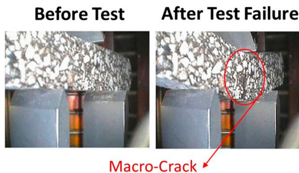
Figure 5. Detail of the crack evolution control performed during the tests.
