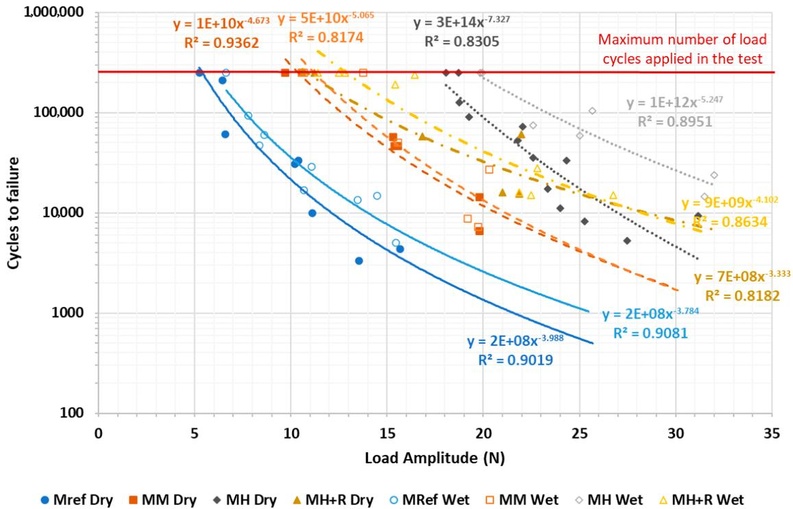
Figure 9. Fatigue laws of the mortars studied in the 3-point bending fatigue test using the DMA.
