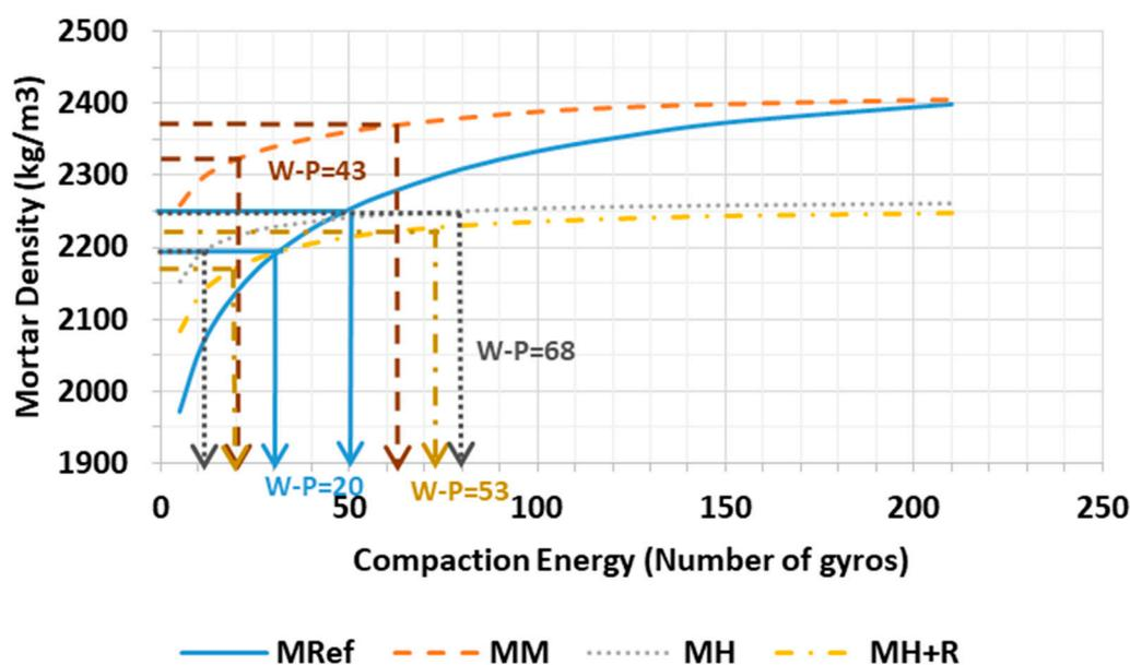
Figure 8. Compaction curves of the mortars studied.
