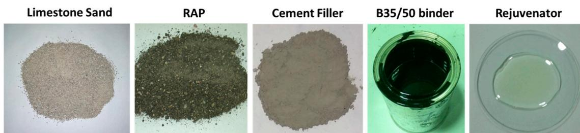
**Figure 1.** Materials used for the manufacture of the mortars studied.
