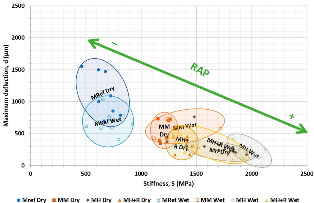
Figure 10. Results of the stiffnesses and maximum deflections measured for the different mortars studied.
