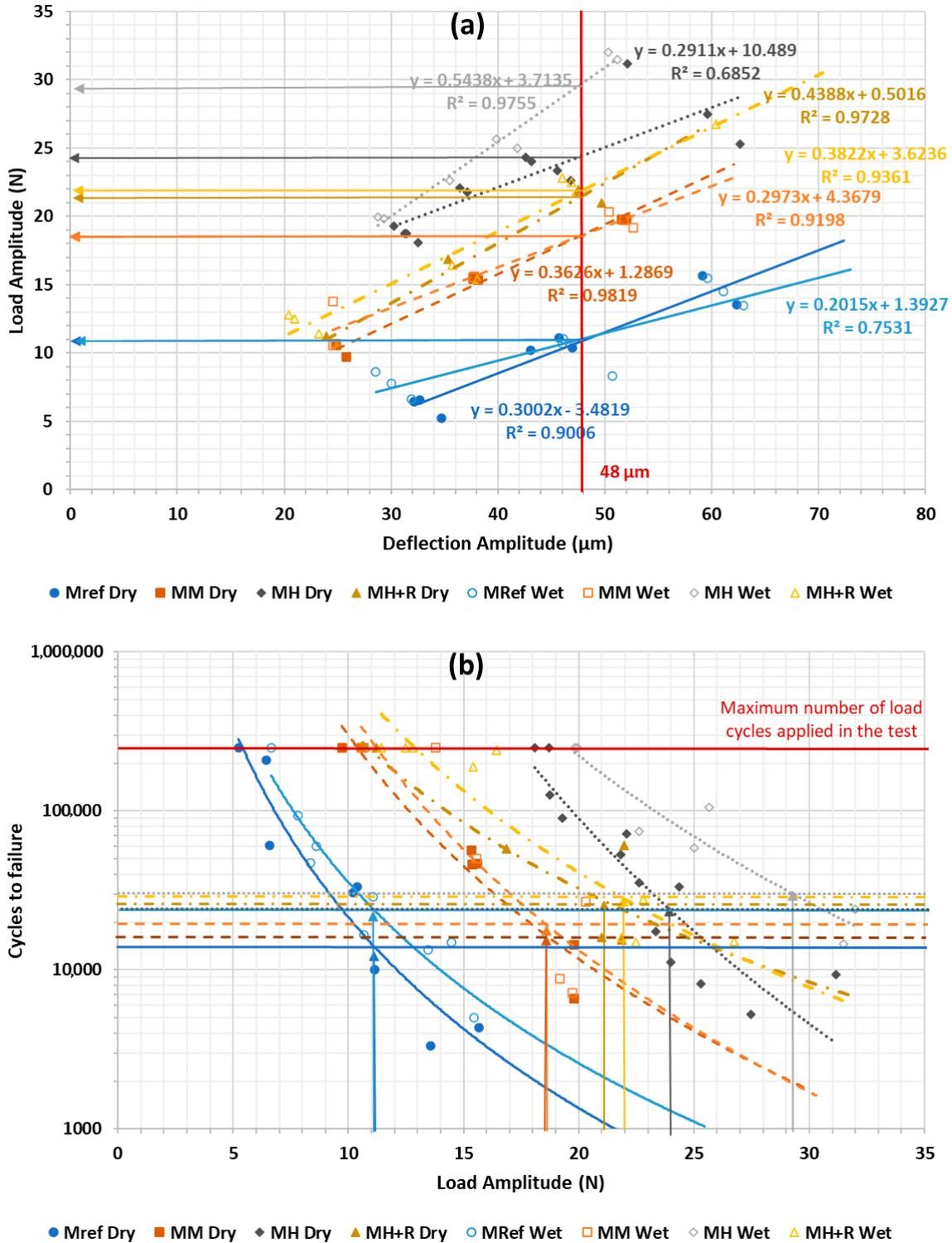
**Figure 11.** Analysis of the mechanical performance of the mortars studied: (a) load amplitude for a given displacement; (b) fatigue resistance for a given load amplitude.
