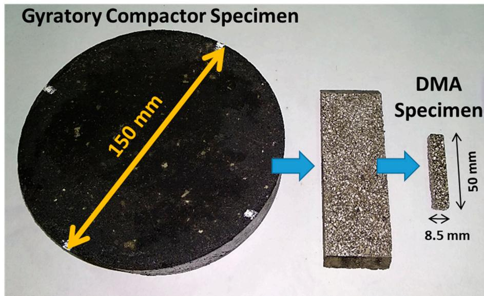
**Figure 2.** Specimens used in the dynamic mechanical analyzer (DMA) tests.
