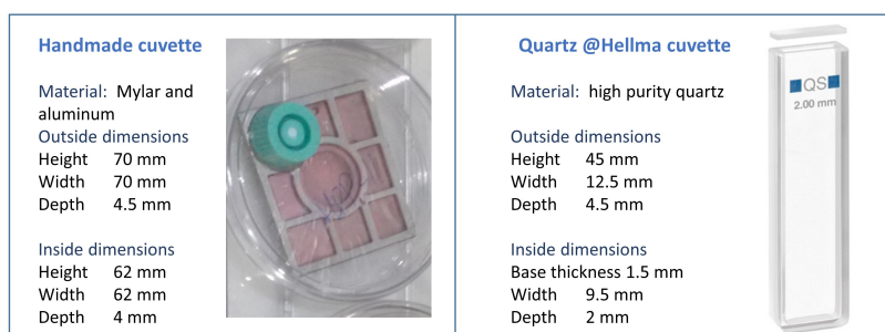
Figure 4.9: Containers for cell irradiation at ILL. Left - a handmade container made in aluminum and Mylar used in the first trials of ILL irradiations. Right - the Hellma quartz cuvettes of 2mm depth, i.e. water layer thickness, that were selected as the final containers for the experiments at ILL.
