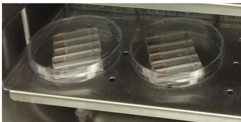
Figure 4.19: Quartz cuvettes with 200 \mu l cell suspension are incubated horizontally inside Petri dishes to avoid contamination. After 12-24 hours incubation, the cells will be attached in one layer in the area covered by culture media.
