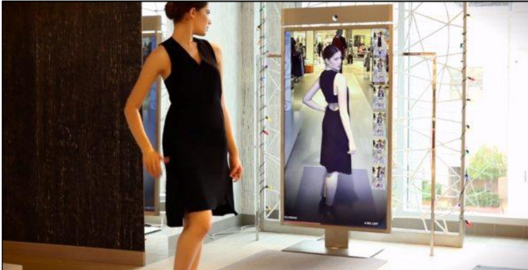
Illustration 9.3 MemoMi MemoryMirror Intelligent Digital Mirror with Intel RealSense Camera, Source: Venture Beat
